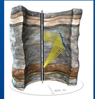
Imaging fractures that do not intersect the well
